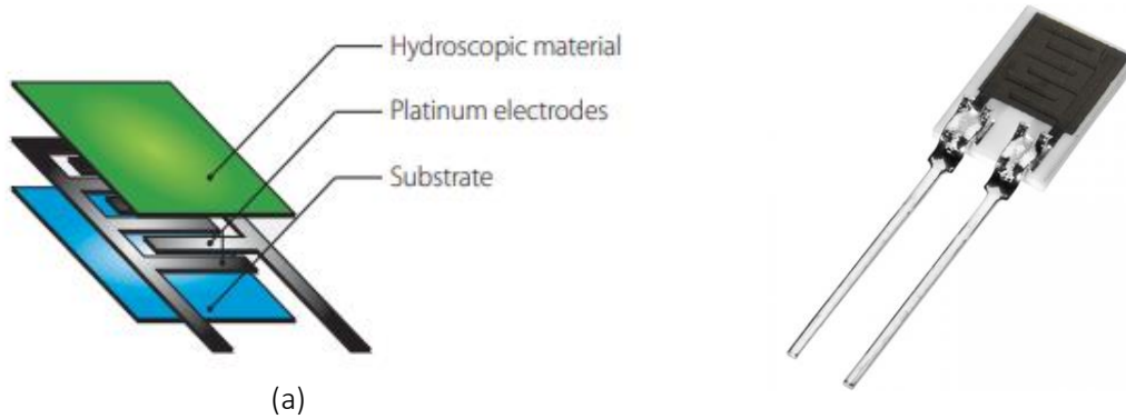
Figure 22: (a) simplified structure of a resistive sensor (image provided by Andivi, ND) and (b) example of relative humidity resistive sensor (model SHS-A4L by bb-sensors)
