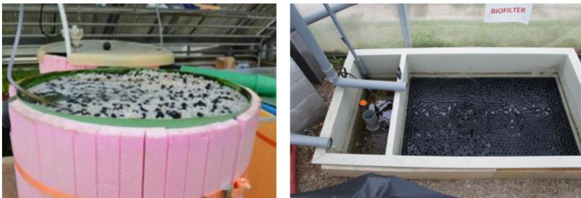
Figure 28: Two versions of suboptimal moving media biofilters: (left) biofilter containing too many biochips (right) biofilter with no aeration (photo: U. Strniša)
